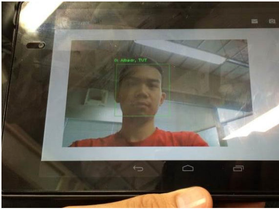
Figure 5. Image result of face detection and recognition which received from server is displayed on portable device
