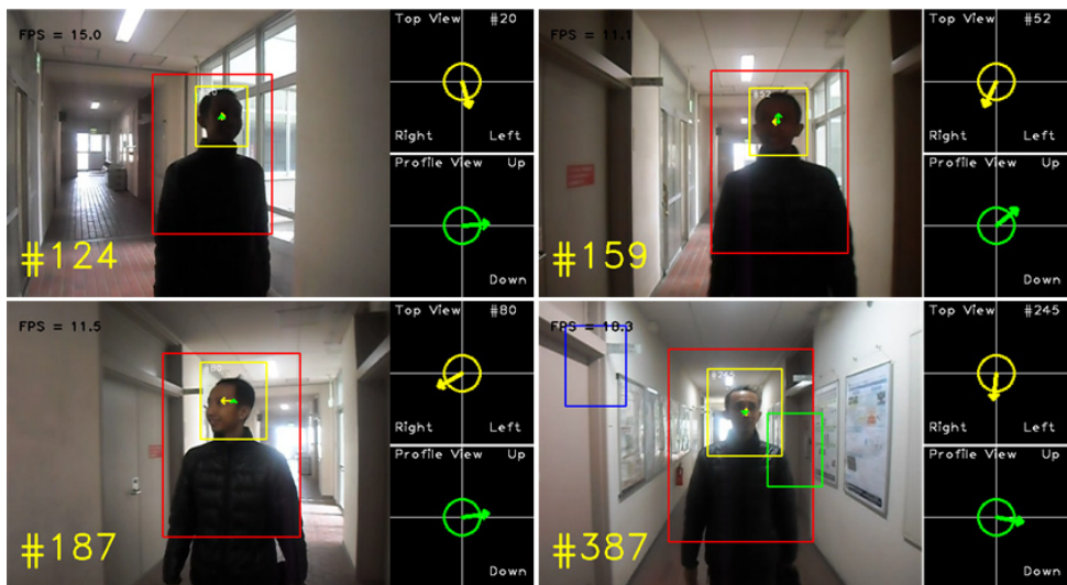
Fig. 14 Experimental results of an online indoor scene. First, the human upper body is detected and tracked (red bounding box). Head detection and head orientation estimation supported by tracking is performed within the body’s bounding box. The estimated head orientation is shown by yellow (pan) and green (tilt) arrows within the bounding box. Miss-orientation estimation (#159) occurs due to a severe illumination, while false positive detections of the human upper body and miss-orientation estimation (#387) occur due to an ambient light and a less fit of the head tracking.
