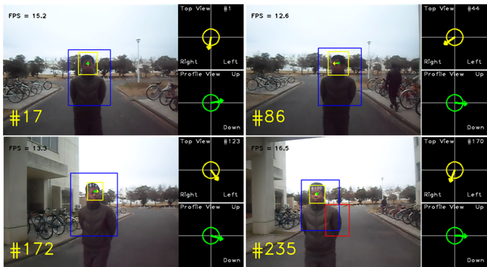
Fig. 15 Experimental results of an online outdoor scene. First, the human upper body is detected and tracked (blue bounding box). Head detection and head orientation estimation supported by tracking is performed within the body’s bounding box. The estimated head orientation is shown by yellow (pan) and green (tilt) arrows within the bounding box. The human upper body detection, the head detection and the head orientation estimation achieve good performances in this experiment.
