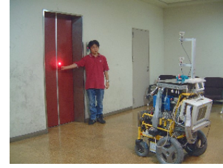
Fig. 12. Teaching the elevator position to the robot.
