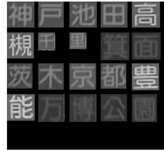
Fig. 19 Template images of characters on guidance signs. These templates are extracted from a videotaped image sequence.
