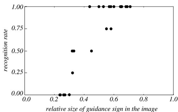
**Fig. 21** Relationship between sign size and recognition rate.**Table 2** Result of on-line guidance sign recognition.
