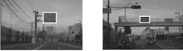
Fig. 10 Detection of guidance sign candidates.
