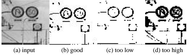
Fig. 3 Binarization results using various thresholds.
