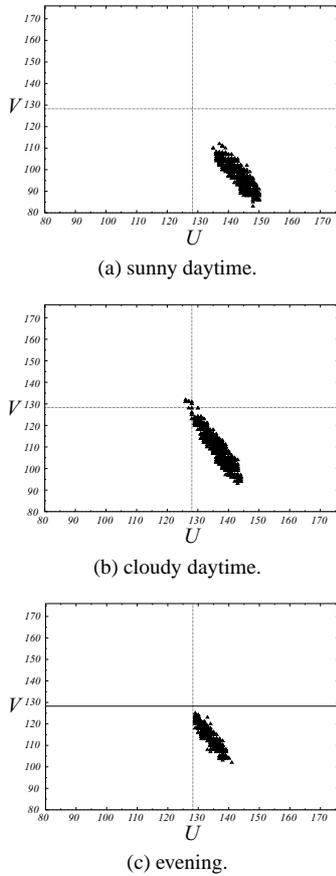
**Fig. 6** Change of color distributions of guidance signs.  $U, V$  values are quantized to  $0 \sim 255$ .  $(U, V) = (128, 128)$  indicates that the saturation component is zero.
