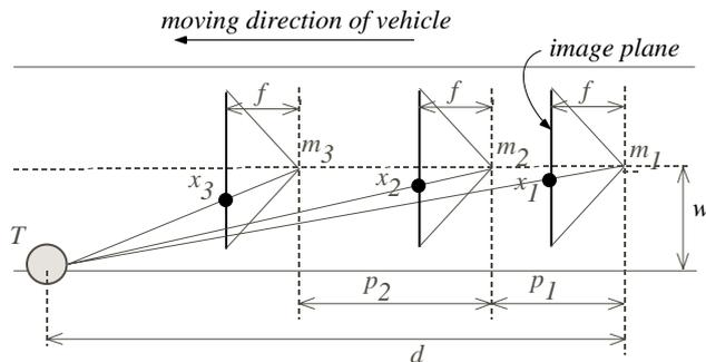
Fig. 11 Predicting target motion.
