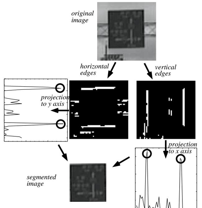
**Fig. 9** Detecting four boundary line segments of guidance sign.
