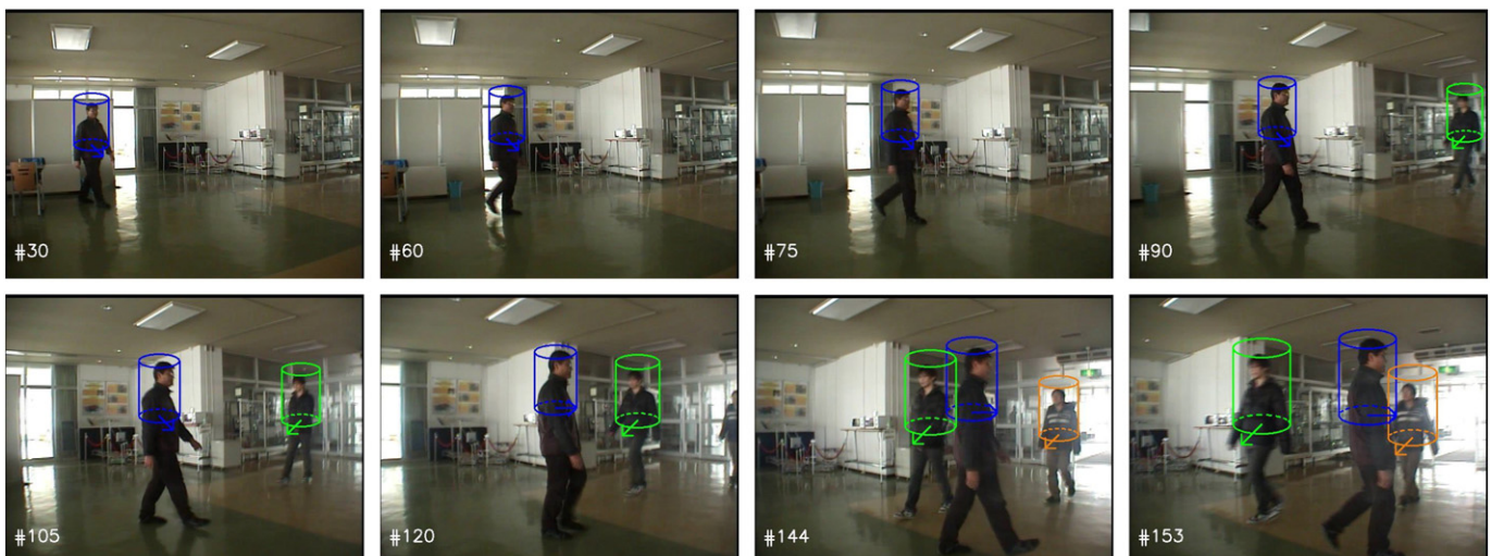
Fig. 13. Human upper body orientation estimation results in the cafeteria with a moving camera.
