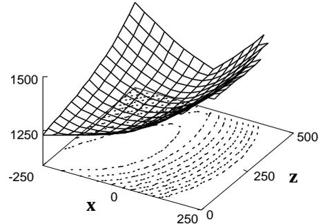
Figure 9: Lower bound of the cost for each observation point which is less than the incumbent value (the cost of the detour in this case). A robot is at  $(-250, 0)$ ; the observed features of the obstacles are at  $(-40, 500)$  and  $(40, 500)$ .
