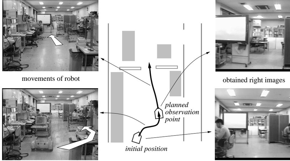
Figure 11: An experimental result: [center] the planned observation point and the trajectory taken by the robot; [lower-right] the right image obtained at the initial position; [upper-right] the right image obtained at the next observation point; [lower-left] the movement from the initial position to the next observation point; [upper-left] the movement from the next observation point into the gate.
