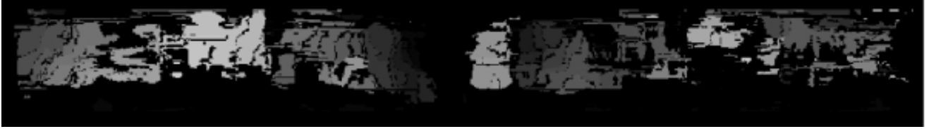
Fig. 5: Panoramic disparity image obtained from the images in Fig. 4. Brighter pixels are nearer.
