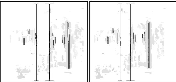
Figure 6: Matching results by the SAD-based stereo matching and fitted boundary edges: Gray regions are matched positions, and black vertical segments are selected matched segments. The long vertical lines are fitted boundary positions, and the positional uncertainties are shown by horizontal lines on the top and the bottom of the position.
