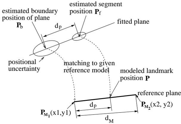
Figure 4: Modeling relative feature position with respect to the boundary position of the reference plane.
