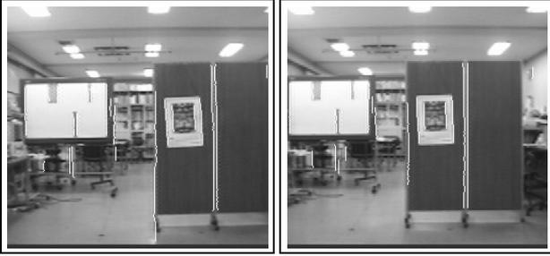
Figure 5: Matched segments by using the segment-based stereo matching.
