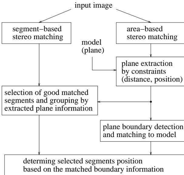
Figure 1: Processing flow of landmark selection.
