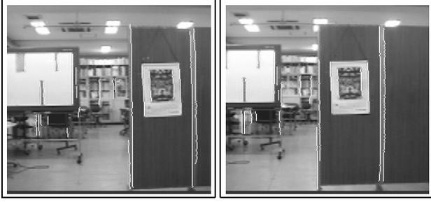
Figure 8: Matched segments by only using segment-based stereo matching: the robot observes five landmarks in the partition plane.
