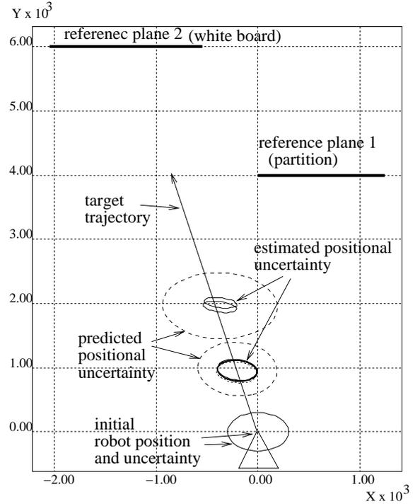
Figure 10: Motion result using on-line selected landmarks.
