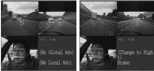
(a) The traffic becomes slow ( t = 121.7 ) (b) The driver is advised to change lane later ( t = 127.3 )
