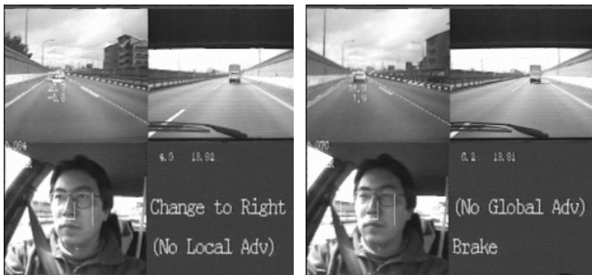
(a) Front vehicle is approaching ( t = 48.9 ) (b) Brake advice is issued ( t = 50.2 )
