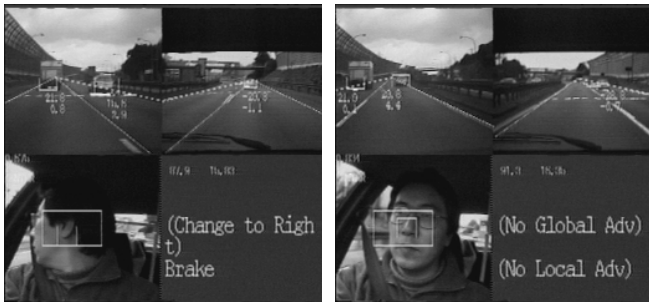
(c) The driver checks the faster lane ( t = 131.9 ) (d) Changing maneuver is executed ( t = 135.3 )
