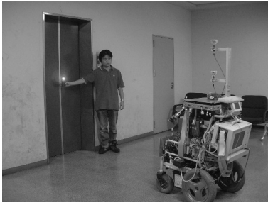
Fig. 7: Teaching the elevator position to the robot.
