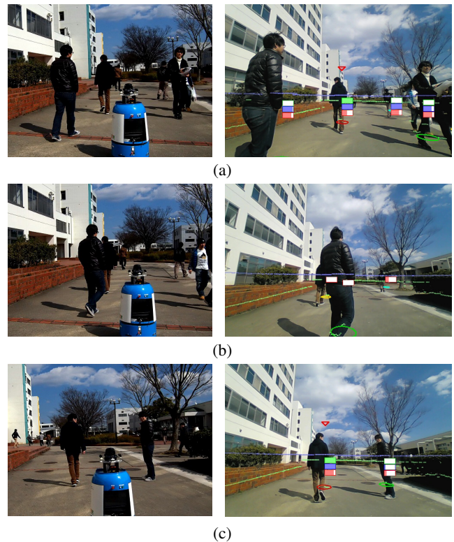
Fig. 9. Specific person following experiment: The left column shows experiment scenes and the right column shows view of the camera on the robot. The meanings of the markers (triangle, circle, bars) are the same as in Fig. 8.
