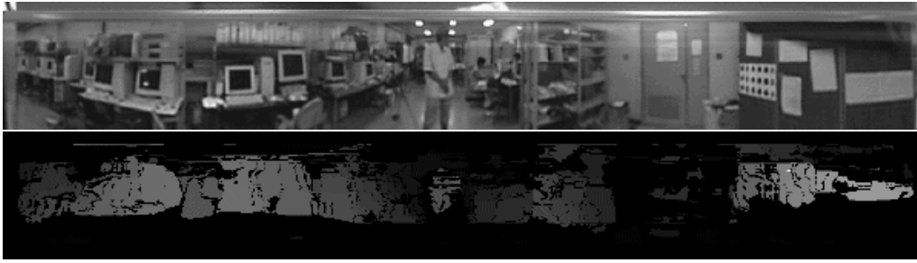
Figure 2: Omnidirectional disparity image. Brighter pixels indicate larger disparities.
