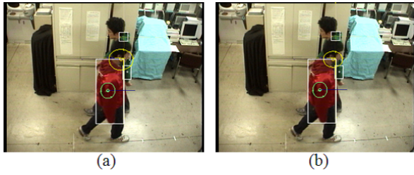
Fig. 3. Comparison of iterative Kalman filter and extended JPDA Kalman filter . (a) Use of iterative Kalman filter . The ellipses show the 99% probability area where the estimated position is located. (b) Use of extended JPDA Kalman filter . The ellipse is smaller. The estimated position is more certain when using the extended JPDA Kalman filter .
