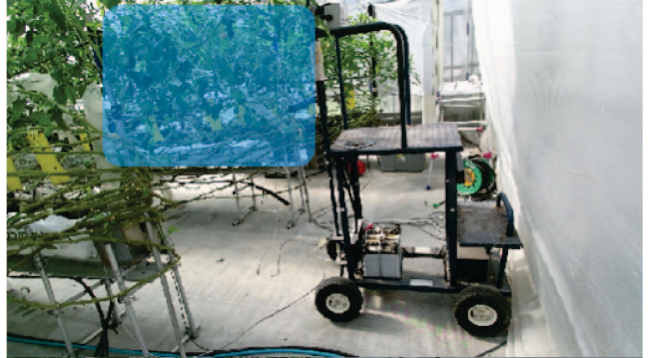
Fig. 4. A path covered by plant in a greenhouse at Toyohashi University of Technology. The region shown in a blue rounded rectangle is covered by the branches spreading out from the cultivation device on the left.
