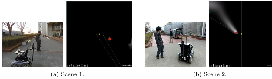
Fig. 6. The probabilistic target existence maps and corresponding scenes. The upward direction in the map is aligned to the heading of the robot. Red boxes in the maps indicate the highest probability cells.
