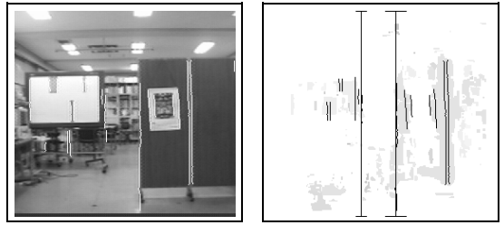
Figure 2: Matched segments by using the segment- and area-based stereo matching, and detected boundary edge positions.
