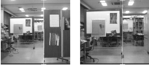
Figure 7: On-line extracted landmarks at the initial position and after 2m motion under normal lighting condition, respectively.
