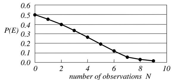
**Fig. 7:** Decrease of the probability of obstacle existence according to the number of observations.
