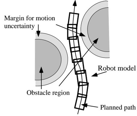
**Fig. 9:** Safety check of a path.
