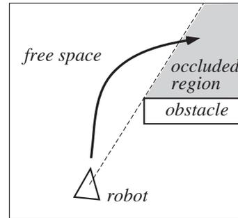
Fig. 7. A robot entering an occluded region.
