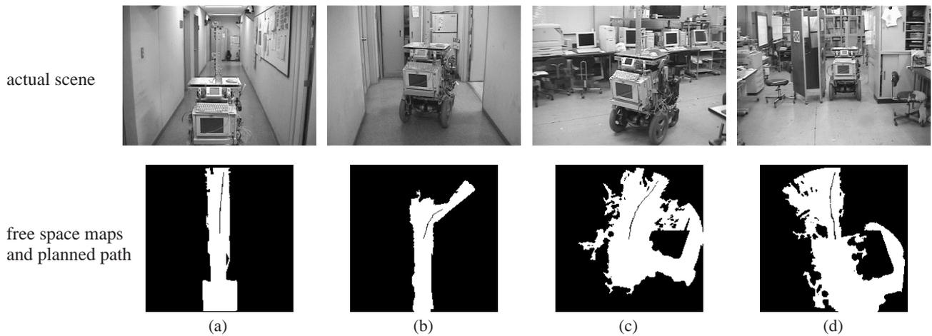
Fig. 16. Experimental results on free space maps and planned path. Black regions indicate obstacles and are expanded by the margins for the motion uncertainty and the robot size in path planning.
