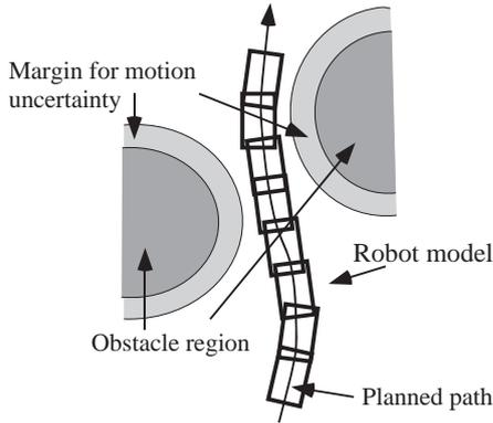
Fig. 11. Collision check of a path.
