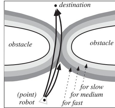
Fig. 12. Path planning for a narrow space with multiple speeds.
