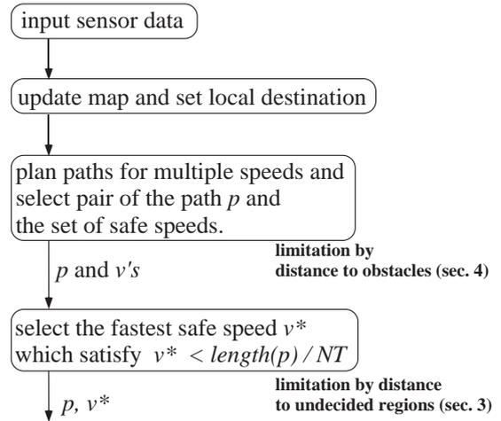
Fig. 13. Flow of speed selection procedure.
