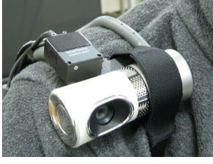
Fig. 1. Interface which has a camera, an orientation sensor, and an accelerometer.
