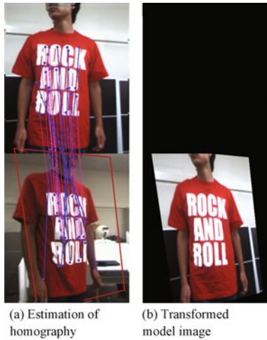
Fig. 9 Estimation of homography by using RANSAC
