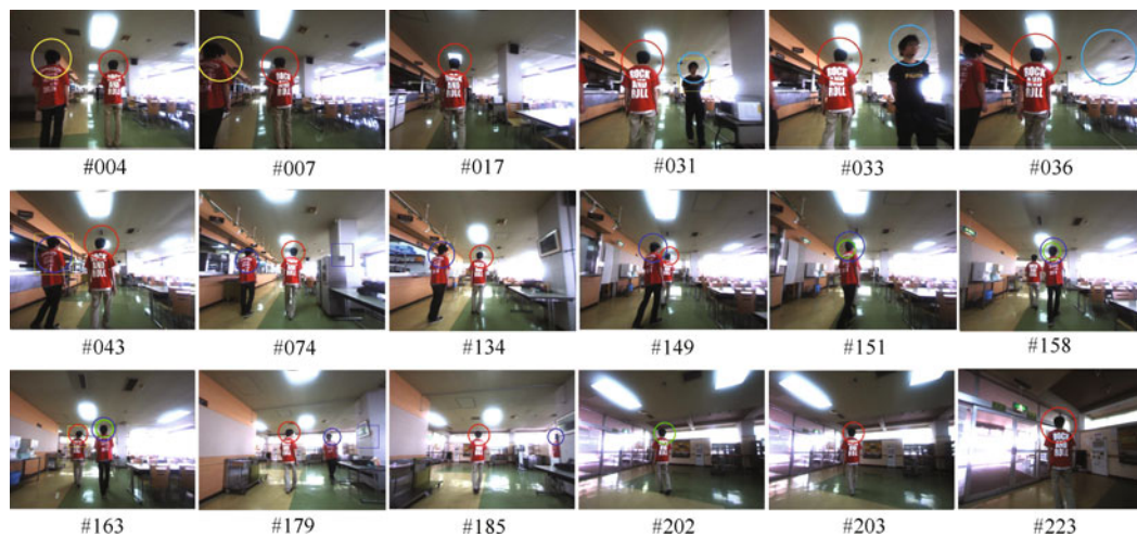
Fig. 20 Experimental result of a specific person following with a mobile robot
