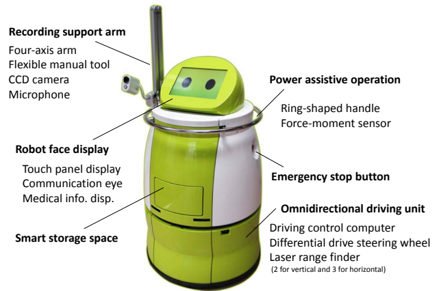
Figure 4. Hardware construction of Terapio
