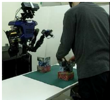
(4) After the advice, the robot asks the learner to demonstrate again. This time, he does it correctly and the belief becomes above the threshold. The robot then judges that the knowledge of this assembly step is correctly transferred.
