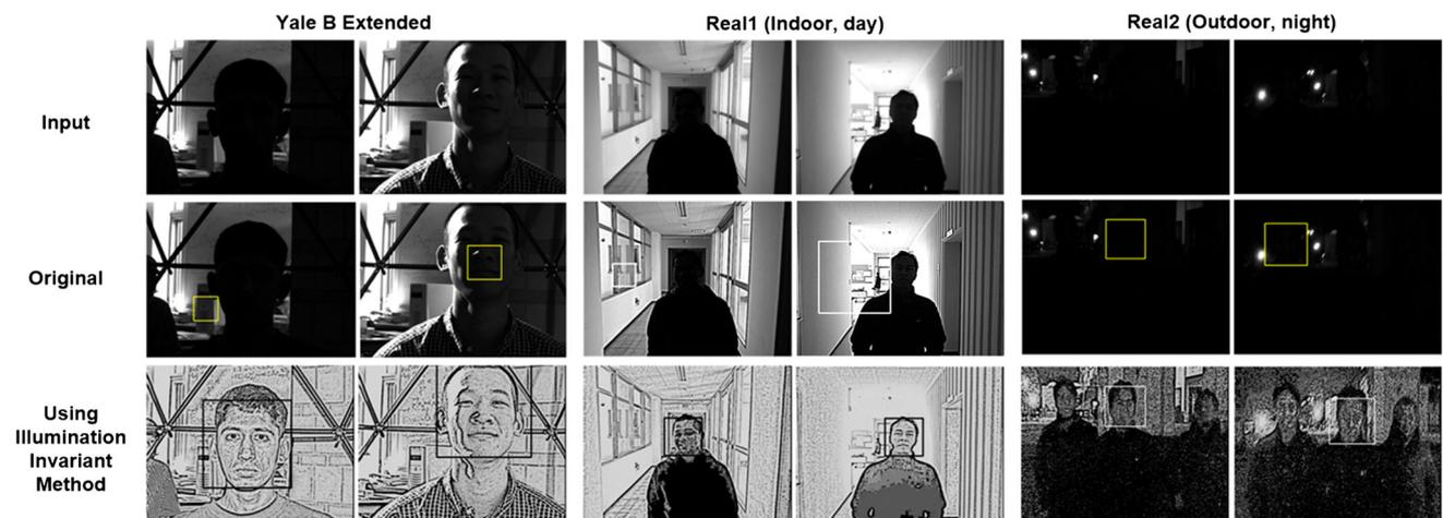
**Fig. 16** Comparison of the performance of face detection without and with the illumination invariant method. Upper images show the input images. Middle images show the face detection results without illumination invariant method. Lower images show the face detection results
