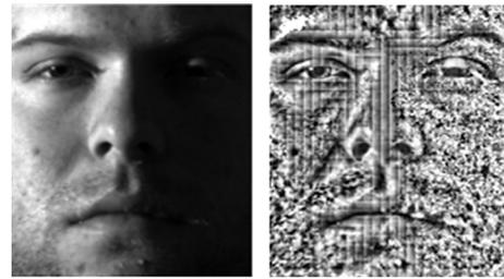
Fig. 5 Block histogram equalization; original image (left), BHE'd image (right)
