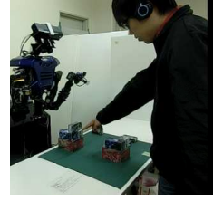
(2) Human asks if blocks 2 and 4 are aligned [i.e., relation coplanar (4-B, 2-C)]. From this query, the robot supposes that the human is ambiguous in this relationship, and calculates the bpa shown in red. Subsets that include consequences with and without that relationship have higher probabilities. Combining this and the bpa above, the bpa in blue is obtained. Since the belief of the correct subset, 0.54, is less than the threshold, the robot plans an interactive action of answering 'yes', and this makes the probability of the correct subset higher.
