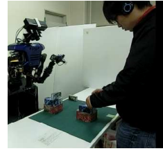
(3) After getting an answer to the query, the learner demonstrates what he has learned. From a combination of prior knowledge with knowledge gained from newly observed demonstrations (in red), the robot gets the blue bpa on the right. Since the belief of the correct subset is higher than the threshold, the robot considers that the learner obtained enough knowledge of this assembly step, and moves to the teaching of the next step.
