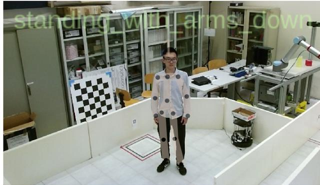
**Fig. 3.** Skeleton joints of a person and the corresponding body pose label, as shown in our system. The upper-limbs pose is recognized as *arms\_down*, and the lower-limbs pose as *standing*. The system provides real-time output.
