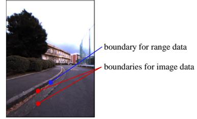
Fig. 3. Gaps between road boundaries for range and image data.
