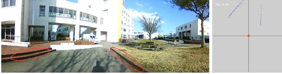
**Fig. 9.** Detection of low steps. A local obstacle map centered at the current robot position is shown on the right. Red ellipses on the left show the detected step locations.
