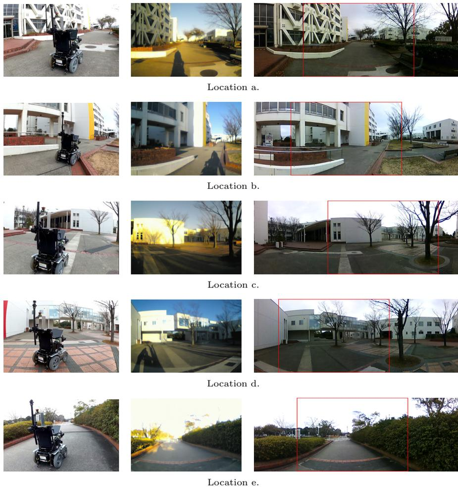
**Fig. 11.** Navigation experiment. Left: Robot in motion. Center: Estimated location (i.e., best matched training image). Right: Input image and selected moving direction.
