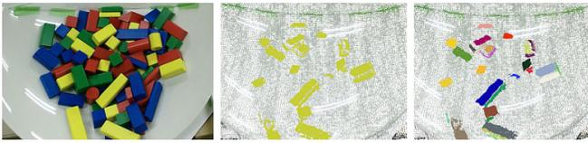
Fig. 6. An example result of color-based pixel clustering and surface detection. From left to right: KinectV2 input, detected only yellow objects, and surface detection result.
