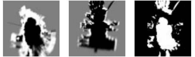
Fig. 7: Probabilistic grid map (left: stereo, center: LRF) and integration result (right).
