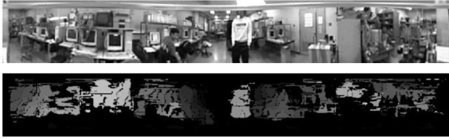
Fig. 2: Omnidirectional stereo (upper: panorama image, lower: disparity image).
