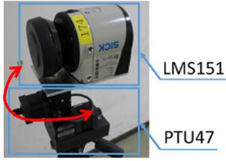
Fig. 1. A 3D scanning system.
